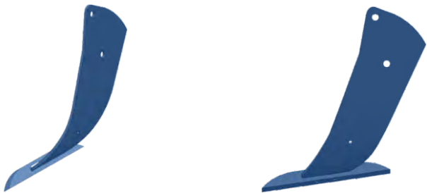
Subsoiler with a deflected Michel type tine, “long” version
