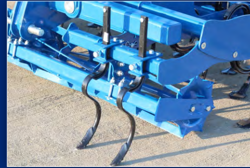
Looseners operating before the basic working elements of the machine
