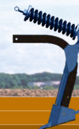
Atlas tine, working elements with built-in cemented carbide
