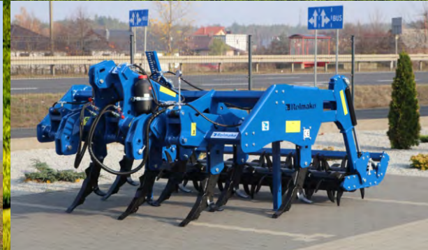
Deep looseners equipped with tines
