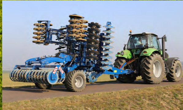
Harrows equipped with tillage discs
