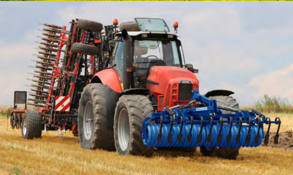
Machines on the tractor front three-point linkage
