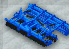
U 652 mounted with a hydraulically foldable frame
