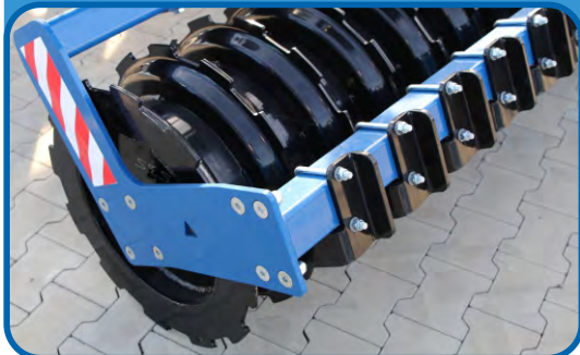
Double Crosskill roller Ø 400 mm + Finisher string roller Ø 270 mm
