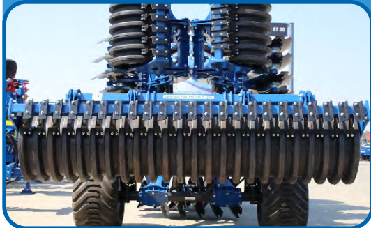
Prismatic roller ORION Ø 500 mm
