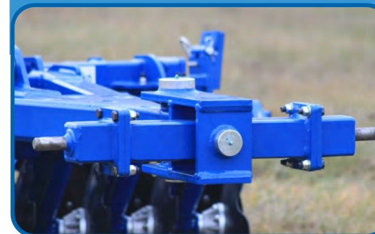
Standard drawbar with a hitching beam
