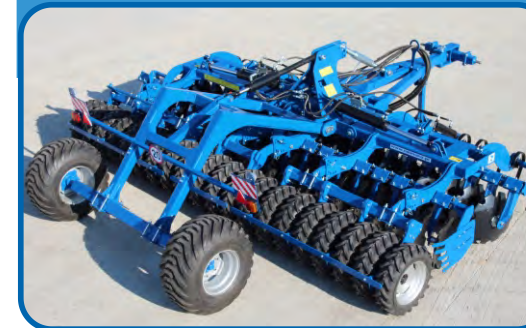
Trailed disc harrow with a tire roller
