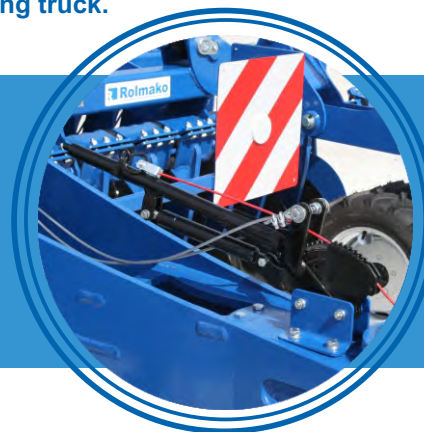
Manual parking lock for the hydraulic brake
