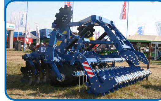
Trailed disc harrow with a tire roller
