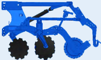
Mounted version with coupler for seeder
